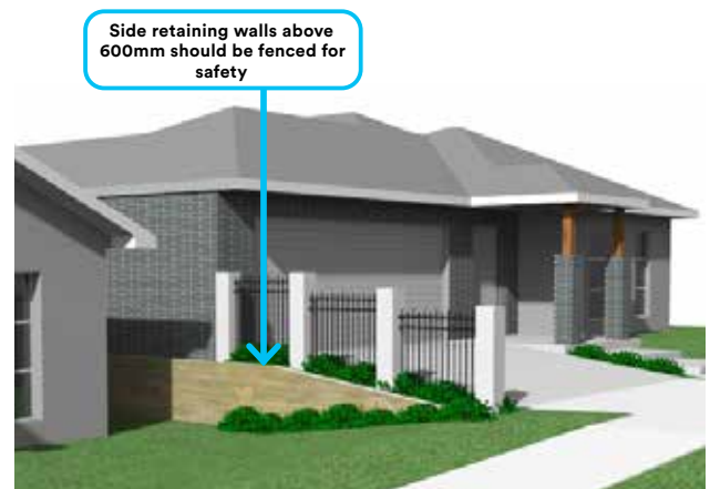
Retaining walls forward of the house
