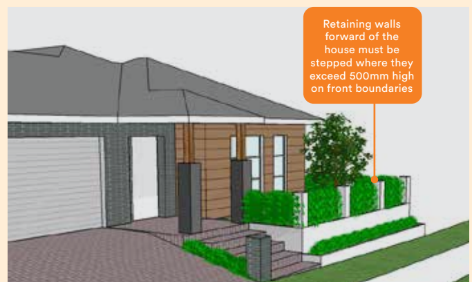
Retaining walls forward of the house
