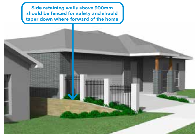
Retaining walls forward of the house
